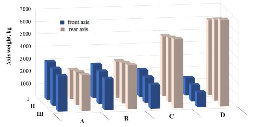
Fig. 4. **Dependence of front adjusting ballast and sprayer mass on axis load** Note: A – tractor axis load without spreader; B – tractor axis weight with empty spreader; C – tractor axis weight with 1000kg fertilizers; D – tractor axis weight with 2000kg fertilizers; I –maximum length ballast position; II – middle ballast position; III – default ballast position
