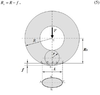
Fig. 2. Deformation of tire
