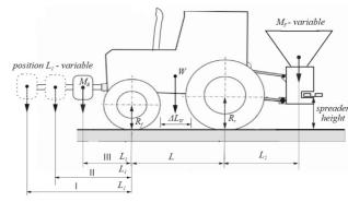
Fig. 3. Measuring of axis weight
